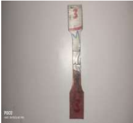
Figure 7 Materials after breaking
