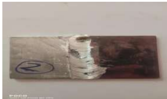
Figure: 5 . Welded butt joint of aluminum and copper
